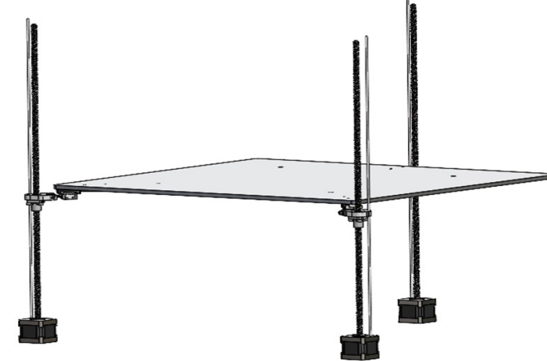
Figure 5. The outer sample tray is fixed to the dancing table whose movements about the x and y axes are controlled by motor-driven lead screws at the two front corners and center of the back edge.
