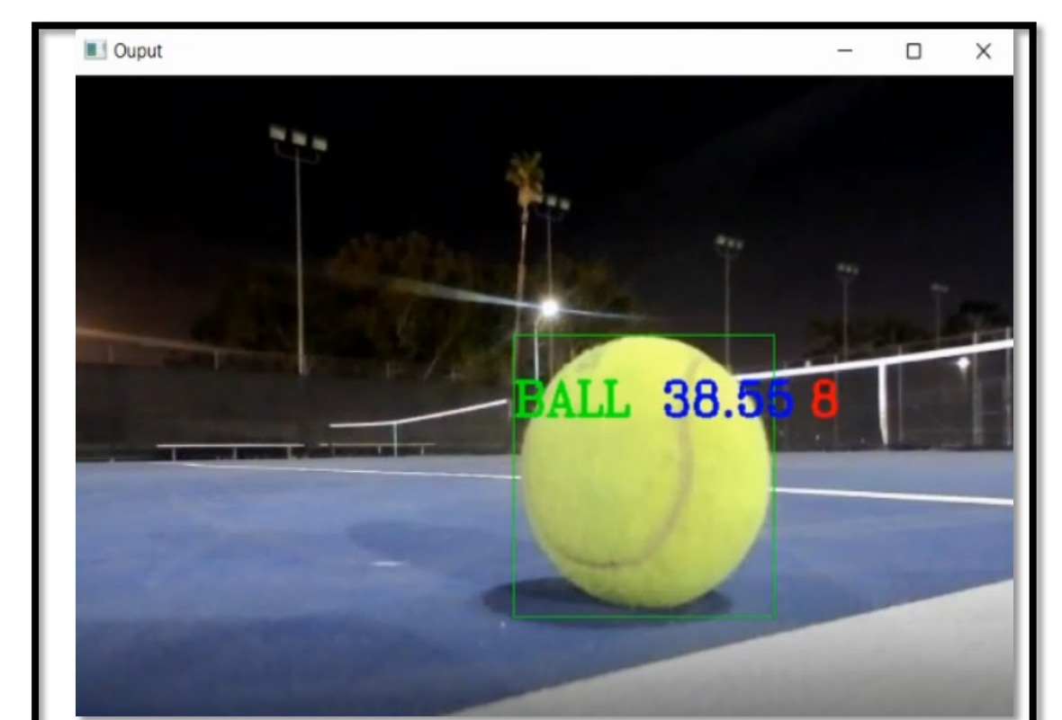
Figure 6. Tennis Ball Detection (BLUE: Confidence Percentage) / Distance Readings (RED: Inches)
