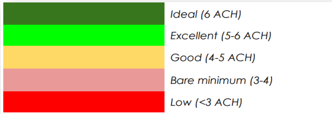
Fig. 2: Air changes per hour and their respective levels of safety. Green being the best, red being the worst. [15]
